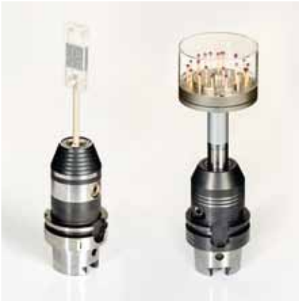
CT inspection items in accordance with VDE/VDI 2630
